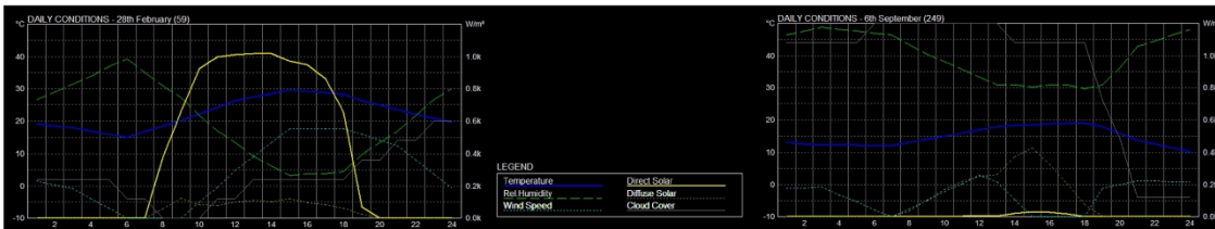
Figure 2 | The graphs above underline the direct solar radiation (Wh/m 2 ) during the hottest day of the year (28 Feb) and the coolest one (06 Sep) in Nairobi, the average of temperature (C°), as well as changes in relative humidity (Calculations with Weather Tool – Ecotect).
