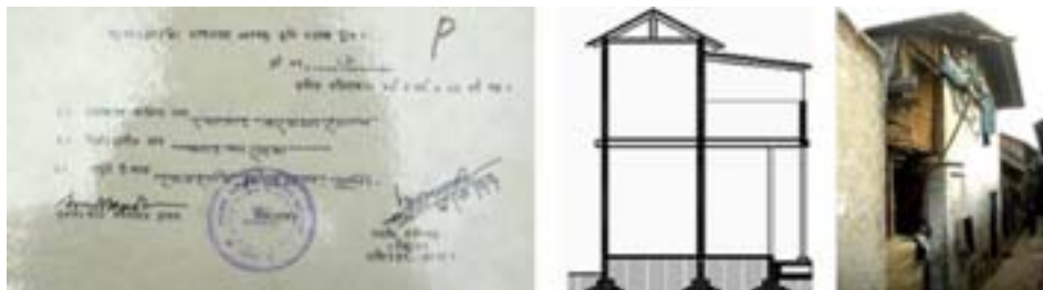
Figure 4. (Left) typical 'Land Allotment Slip' for Vastuhara; (middle and right) brick-built house with wooden floor and CI sheet roof., Source: Author.
