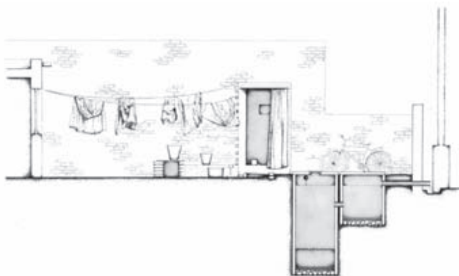
Figure 1. Section through an individual septic tank toilet system constructed in a household yard.
