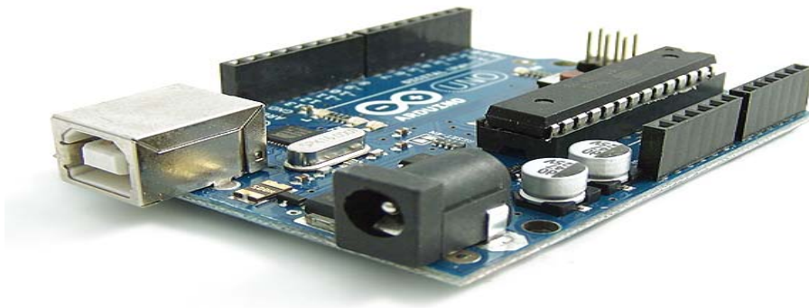
Figure 6. “Arduino” is a simple-to-use open source hardware platform able to integrate with the environment in which it is placed and receive information from a wide range of sensors
